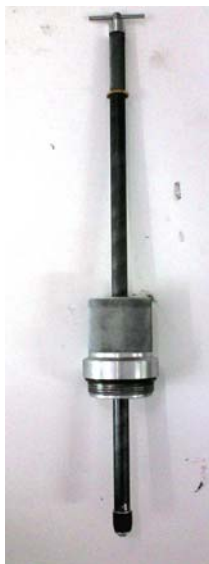
Expansion plug removal / insertion tool.
