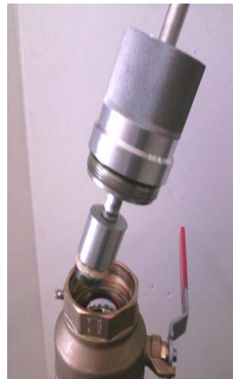
Plug removal tool travels through ball valve to remove plug.
