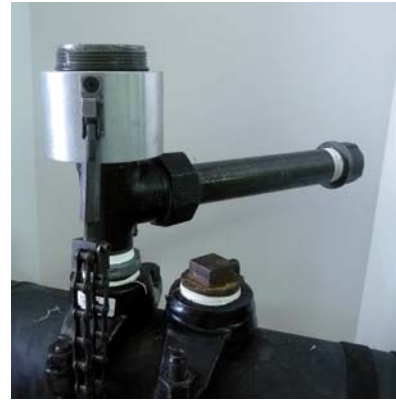
Threaded cap housing attached with chains.
