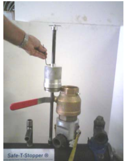
Measure expansion plug insertion depth using collar.
