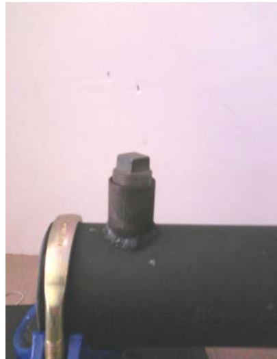
A malleable plug is tightened into the welded coupling.
