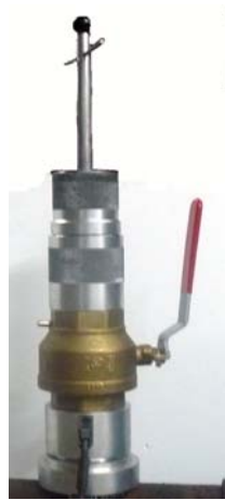
Attached ball valve and extension housing. Plug removal tool will be used to extract tee out of the main.
