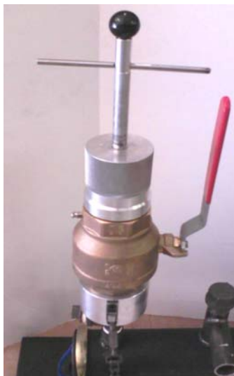
Plug removal tool attaches to ball valve.
