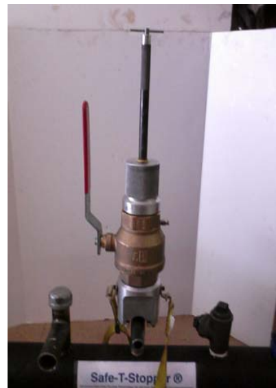
Insert expansion plug below branch to stop the flow of gas.
