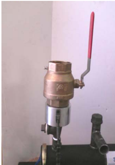
Ball valve attaches to cap housing.
