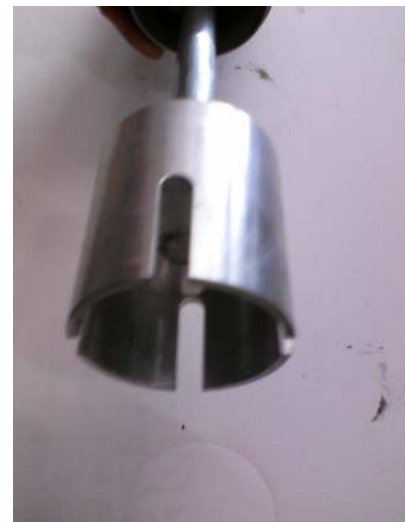
Mueller cap removal/ insertion tool has four keyway slots.
