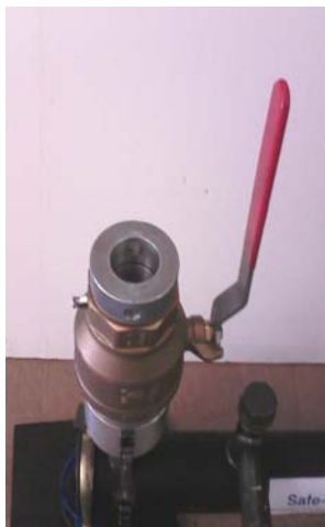
Check expansion plug is properly seated.
