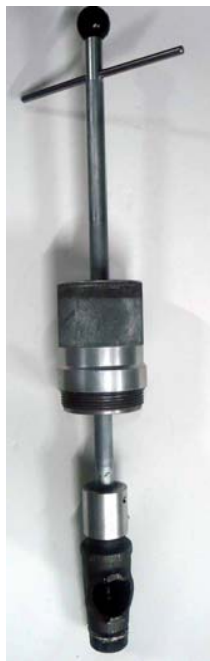
Place cap housing over aluminum adapter and chain the assembly to the main.
