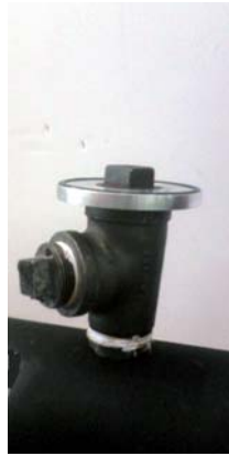
Aluminum disc with embedded o-ring.
