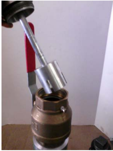
Insert Mueller cap removal tool.
