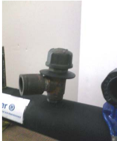
Install first beveled o-ring beveled side down.
