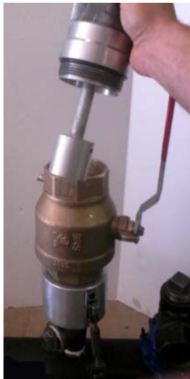
Install ball valve and remove cap with cap removal / insertion tool
