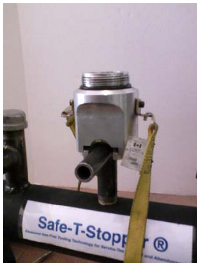
Fit second beveled o-ring with bevel facing up.
