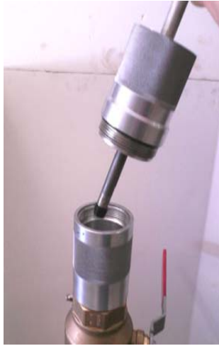
Attach tapered threaded weld plug tool assembly.
