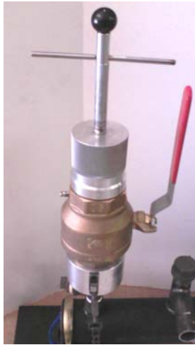
Open ball valve and insert tapered threaded weld plug.
