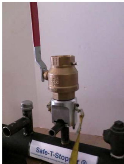
Fit two half collars under beveled o-rings
