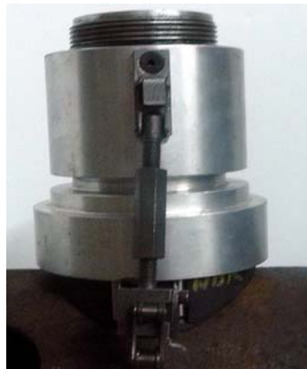
Before cutting off branch tighten plug and loosen tee. Plug should be tighter than tee. Cut branch.
