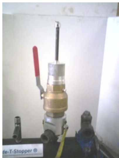
Insert expansion plug below branch to stop the flow of gas.
