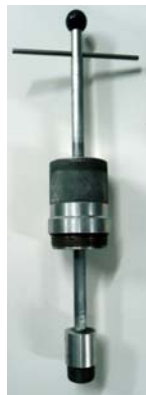
Once tee is removed, replace threaded hole in main with malleable plug using the plug insertion / removal tool.
