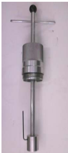
Plug removal tool attaches to shaft.
