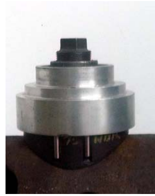
Place aluminum adapter over saddle.
