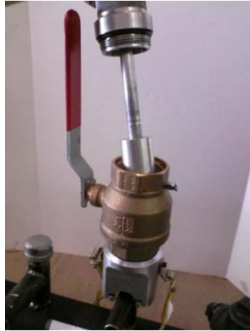
Cap removal tool is attached to ball valve.
