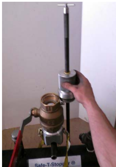
Measure expansion plug insertion depth.
