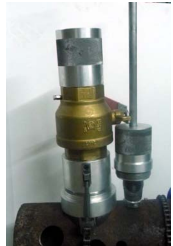
Remove tee and close ball valve.
