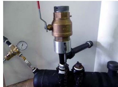
Threaded cap housing attached with chains.
