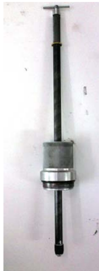
Expansion plug removal / insertion tool.
