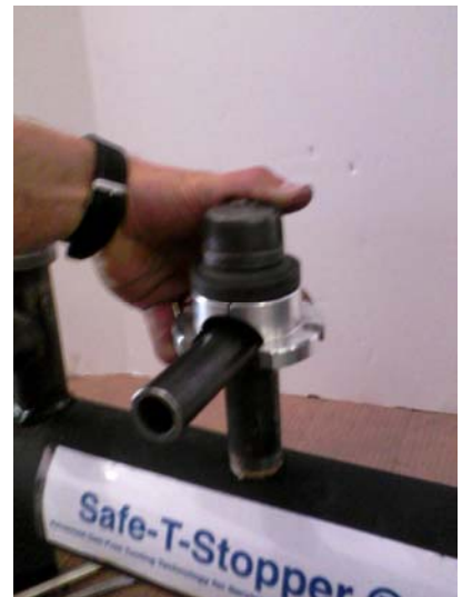
Fit two half collars under beveled o-rings
