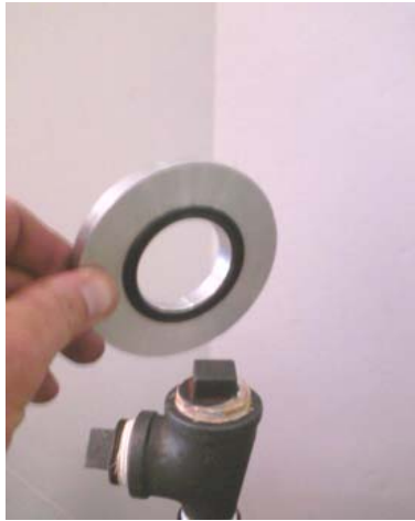
Aluminum disc with embedded o-ring is placed on boss of tee.
