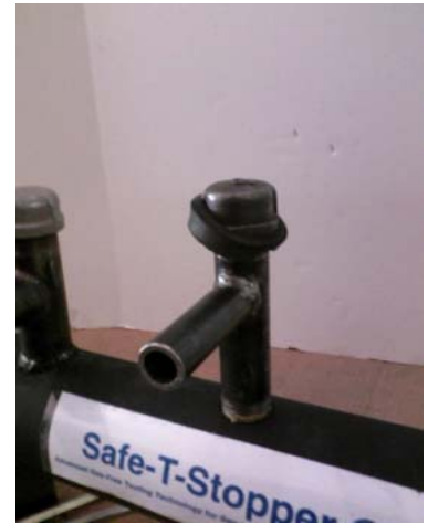
Fit one beveled o-ring with bevel facing down.
