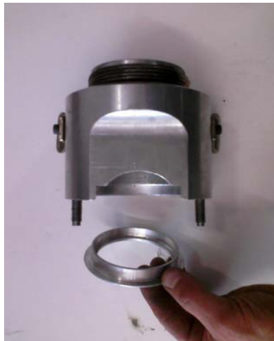
For some tee sizes it is necessary to place reducer ring inside cap housing to achieve gas tight seal around tee.
